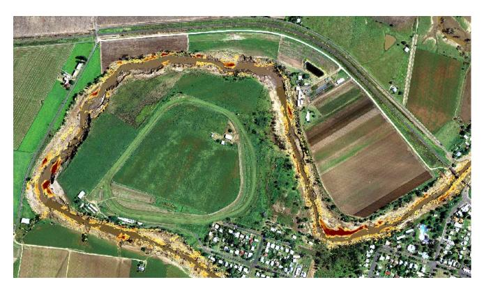
Figure 2. An aerial image of a meander bend from the Lockyer Creek after the 2011 flood. Fluvial entrainment was calculated from differencing the 2010 and 2011 DEM and then highlighted. The darker the colour the greater the volume of erosion in that  $1 \text{ m}^2$  pixel. The volume of mass failures has been excluded from the image for clarity.
